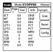
The first page is filled with some of the most common, basic engine parameters, from temperatures & ignition advance, to fuel trims & O2 sensor values.
